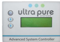
The ROC-5 is a state of the art RO system controller built integral of each system. This controller will enable automatic operation year round. System will automatically turn on when pressure in storage tank is below 40psi. During operation clean water will be produced filling water storage tank. When pressure reaches 60psi the system shuts down. System cycles on-off automatically to maintain between 40-60psi in storage tank.
