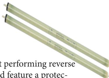
**Test Information:** 550 TDS Filtered (5 Micron), De-chlorinated, Municipal Feed Water, 77°F, 15% Permeate Recovery, 6.5 - 7.0 pH range, at the specified operating pressure. Data taken after 30 minutes of operation. Maximum pressure drop for each element is 15 psi. Minimum salt rejection is 96%. Permeate flow for individual elements may vary +/- 20%.
